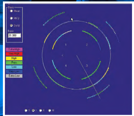
Plot Screen - As the propeller is being scanned, dynamically display results for each measured blade radius. The resulting color coded map provides the technician with an overall view of how the propeller geometry conforms to the specified tolerance, what blade sections are out of tolerance, and by how much.
